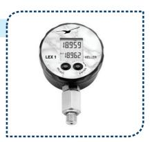
LEX 1 has two operating keys. The left key is to turn the instrument on, to select the functions and the pressure units. The right key executes the selected function resp. unit or serves to display the Max.- and Min.-value
